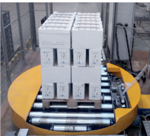
J2000 turntable wrapper integrated in system
